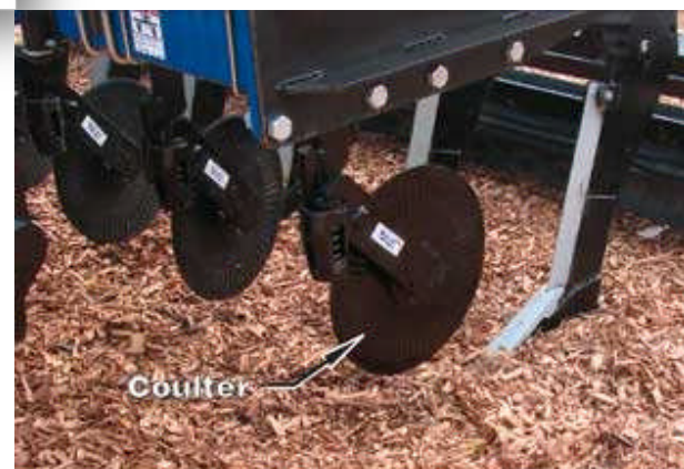
Figure 6. Coulters make narrow slits in top soil
