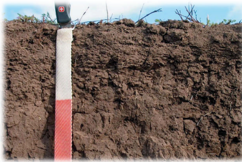
Figure 5. Top layer of soil showing signs of compaction
