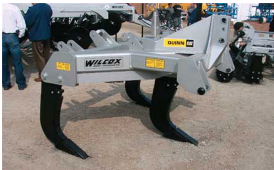
Figure 8 —A three-shank subsoiler which attaches to a tractor's three-point hitch.
