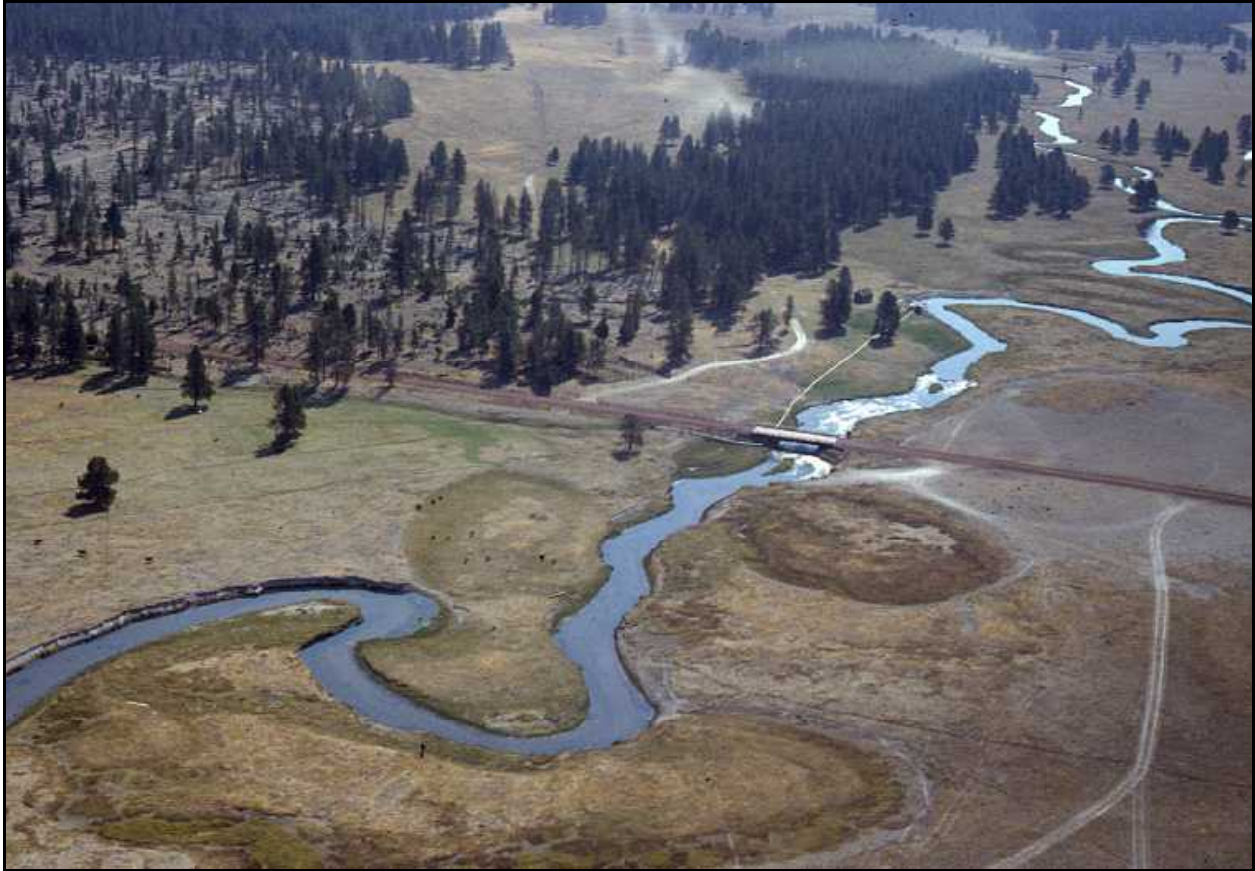
Photo 8-8. View of Upper Williamson River at Rocky Ford Channel incision is more pronounced downstream (left side of picture) of the bridge.
